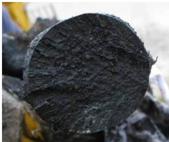
Figure 3. Typical Broken Bar
